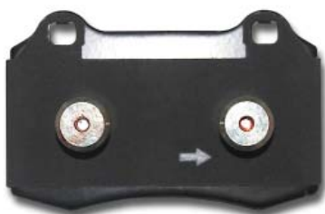
The arrows should follow the direction of disc rotation.
