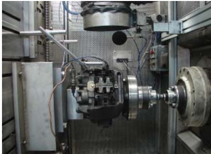
Brake assembly unit being tested inside a sound booth.
